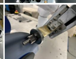
From simple to complex parts, OB7 robotic deburring removes inconsistency and drudgery. Speed, number of passes, and over 360 degrees of rotation can all be applied with ease, and with 7 axis, OB7 can maneuver to suit more complex shapes.
